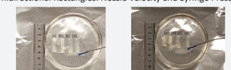
Figure 4. Images of actuated LCEs at 107° C (left) and 116.3° C (right) printed at 30.2 mm length using a unidirectional print path. a) and c) Nozzle velocity of 100 mm/min and syringe pressure of 10 psi. b) and d) Nozzle velocity of 500 mm/min and 20 psi
